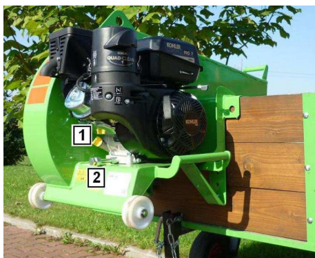
1 – Filler plug and dipstick 2 – Oil filter
